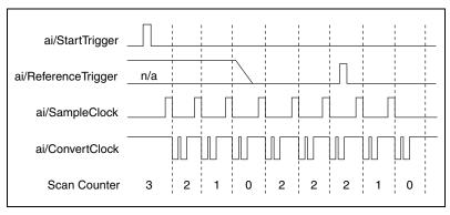
Figure 4-10. Pretriggered Data Acquisition Example
